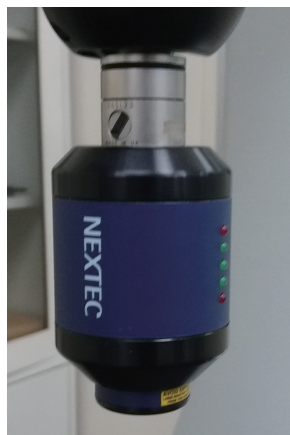
图3 激光扫描测头 WIZprobe Fig.3 Laser scanning sensor WIZprobe
